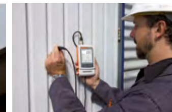
Measurement of a paint coating on steel
